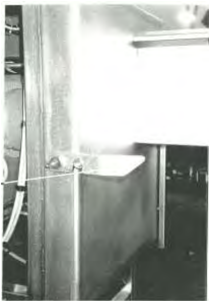
Verrou de carter couteau fermé / Case bolt – closed knife.
