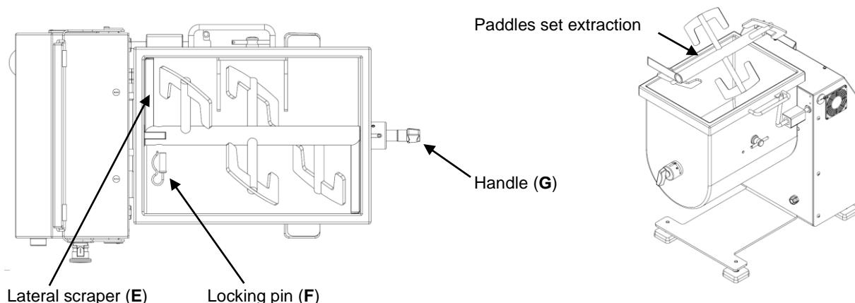
The cleaning will thus be easier. Use hot water, neutral soap and some pieces of cloths. It is also possible to clean the tank and the paddles with a pressure cleaner. Be sure not to apply pressure water directly into the areas around the right and left axles, where the grease seal rings are located.
